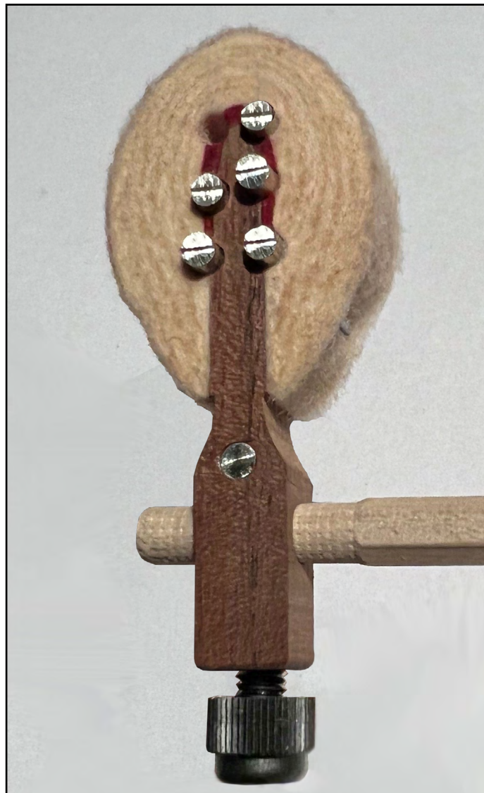
Photo 2: Test hammer with 5 lead-free soft metal inserts for a C4 hammer weight scale #9.
